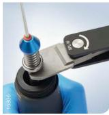
Step 3: Connect the nose cone to the transducer.
