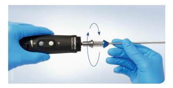
**Step 2:** Place the torque wrench on the probe flats and then turn in the direction of the arrow until the wrench "clicks" to ensure adequate coupling.
