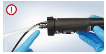
**Step 7:** Adjust the suction control wheel so the marker is approximately at the halfway point of the suction indicator and make sure the hole isn't accidently covered by your finger (causes full suction).
