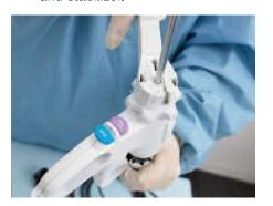
6 For disassembling the instrument and transducer, use the torque wrench to turn the rotation knob counterclockwise while holding the stabilizer.
