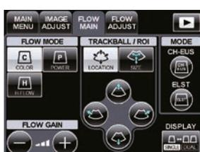
Adjusts the sensitivity of the flow signal in FLOW mode in 32 steps.
