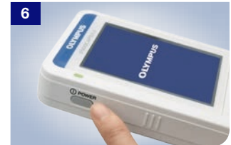
6. Press "POWER" for at least 1 sec. Patient ID and name are displayed on the upper left screen.
