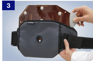
3. Insert antenna sheet into the cover. Orange colored lines printed on the surface should face front. The cable always stays on the patient's left side.
