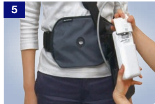
5. Attach the recorder holder on the left side of the patient's body. Connect the recorder and the antenna unit. Slide the connection part until it clicks.
