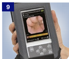
9. Press "MENU" and select "Real Time View". Confirm that images from the body are being received properly. If necessary, images can be played back or captured.
