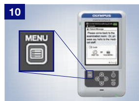
10. Lock the button operation. Go to "Patient Message" and press "MENU" for at least 2 sec. When patient guidance is activated, the patient does not necessarily need to touch the recorder. Beep or vibration will stop after 30 sec.
