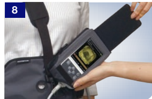
8. Press "MENU" and select "Real Time View". Confirm that images are received properly.
