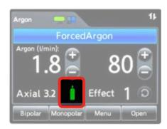
2.) Confirm supply connection indicator displays connection and tank status
