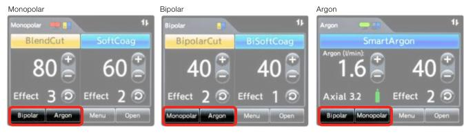
Select mode by tapping on the desired mode located on the bottom of the touch screen
