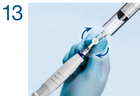
Apply suction by turning the stopcock to the parallel position.
