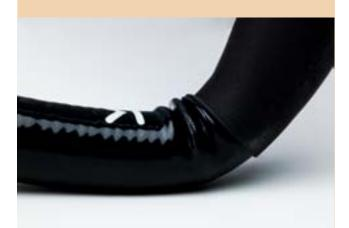
Avoid bending insertion tube within 10 cm from junction of the boot of the endoscope
