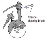
Brush the suction cylinder and the instrument channel port
