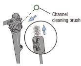
Brush from the suction cylinder to the endoscope connector
