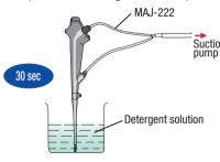
15 Completely immerse the endoscope and the suction cleaning adapter (MAJ-222) in the detergent solution
