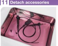
Detach the accessories while keeping the scope immersed in detergent solution. Leave all components to soak in the solution.
