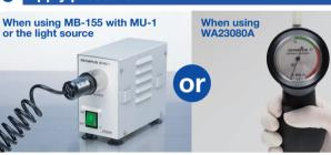
Press the hand pump so that the pointer stays within the green area.
