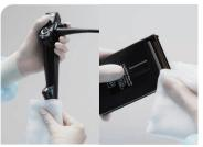
Using a sterile, lint-free cloth, thoroughly and gently wipe and dry the external surfaces of the endoscope.
