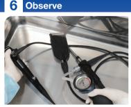
Immerse the entire endoscope in water, observe for 30 seconds or more while angulating the bending section and confirm that there is no continuous series of bubbles. CAUTION : If a leak is detected, remove from water and contact Olympus.
