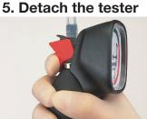
Remove the endoscope from the water and release the air pressure in the endoscope.\* Detach the leakage tester from the endoscope.
