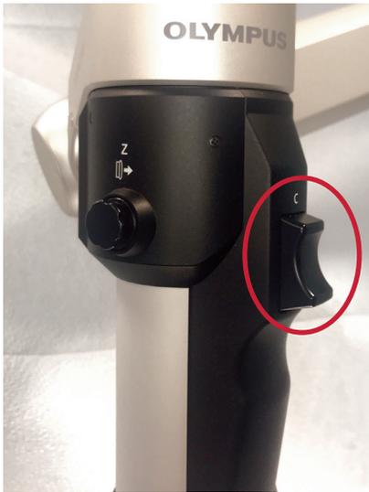
Trigger Brake Release Pull To Move Release to Lock
