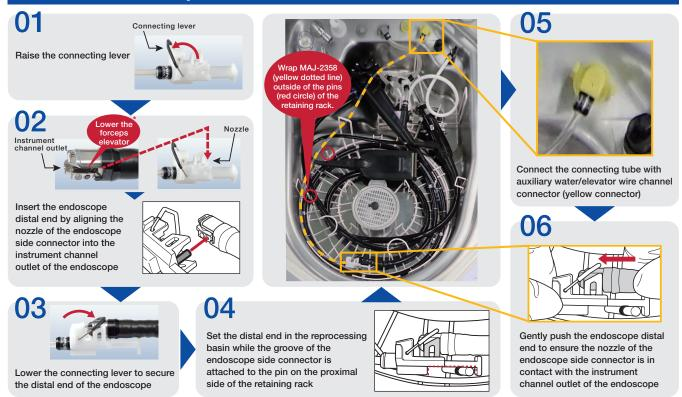
There are some versions of OER-Pro/OER-AW IFU that instruct to raise the forceps elevator to an angle of approximately 45° when reprocessing endoscope which has a forceps elevator in OER-Pro/OER-AW. However, be sure to lower the forceps elevator when reprocessing the endoscope with the MAJ-2358 in OER-Pro/OER-AW
