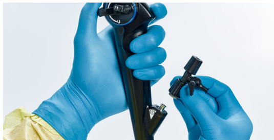
Disassembled MAJ-891 (Forceps/Irrigation Plug)
