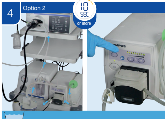
4 Option 2 Alternative method of Step 4 : Use OFP-2 to flush the auxiliary water channel with water for a minimum of 10 seconds, with maximum flow rate.
