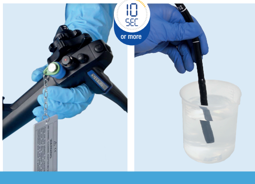
4 Attach AW channel cleaning adapter. Depress the button of AW channel cleaning adapter to flush the air channel with water for 10 seconds or more.
