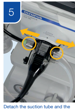
5 Detach the suction tube and the water container's metal tip from the endoscope, then detach the endoscope connector from the video system centre.
