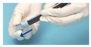
While pressing the button, push in the handle to confirm that handle operation is easy.
