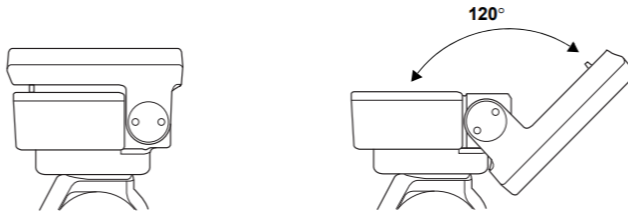
The LCD display tilts by 120 degrees.
