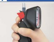
Remove the endoscope from the water and release the air pressure in the endoscope.\*
