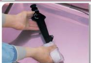
Using a lint-free cloth, gently wipe all debris from the endoscope's external surfaces. while the endoscope is immersed in detergent solution. Soak in detergent solution for the recommended time.
