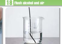
Attach a syringe filled with alcohol and flush three times. Inject air three times.
