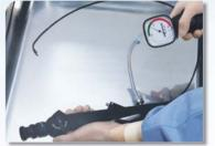
Immerse the entire endoscope in water, observe for 30 seconds while angulating the bending section and confirm that there is no continuous series of bubbles.
