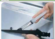
Attach a syringe and flush deionized water three times and inject air three times.
