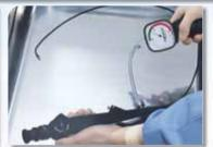
Immerse the entire endoscope in water, observe for 30 seconds while angulating the bending section and confirm that there is no continuous series of bubbles.
