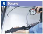
Immerse the entire endoscope in water, observe for 30 seconds while angulating the bending section and confirm that there is no continuous series of bubbles.
