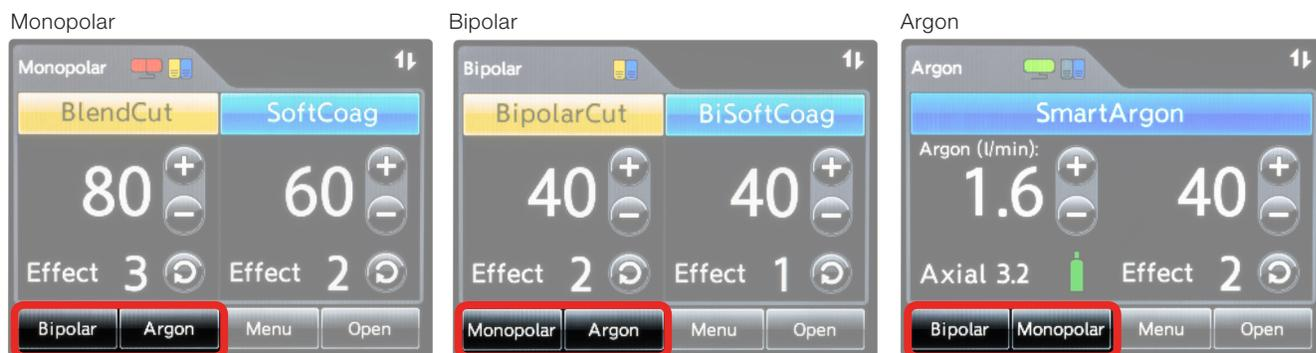
Select mode by tapping on the desired mode located on the bottom of the touch screen
