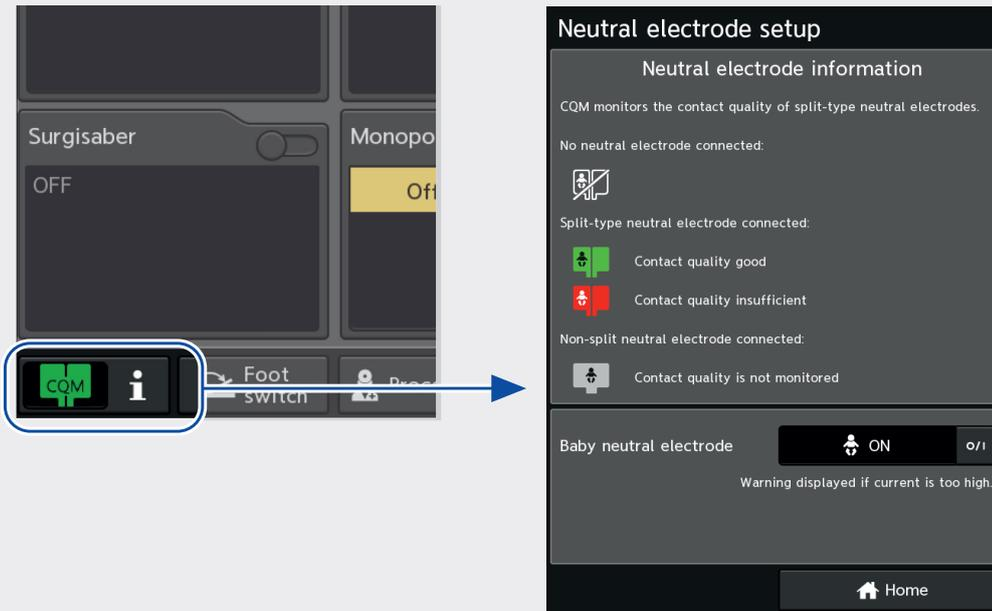
Contact quality will be shown for split type/dual pad neutral electrodes. Contact quality is not known for non-split type/single pad neutral electrodes and won't be indicated.
