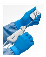
Ensure the tip of the blade is all the way in the bend fixture with the correct window orientation. After bending, the cutting window should end up on the concave side of the blade shaft.
