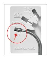
6 Inspect the entire device after bending the blade to ensure the device was not damaged during bending.
