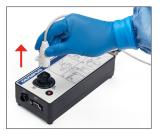
Grasp the malleable device handle with one hand and place the distal tip of the blade fully into the desired angle position as marked on the bending fixture.
