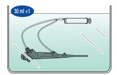
17 Aspirate the detergent solution (through the balloon channel)
