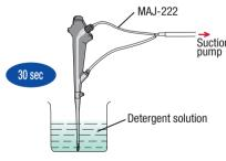
15 Completely immerse the endoscope and the suction cleaning adapter (MAJ-222) in the detergent solution
