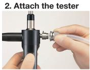
Attach the leakage tester to the venting connector on the endoscope.
