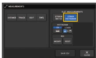
Displays a frequency distribution graph for strain in the set area.
