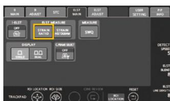
2. Press the STRAIN RATIO button on the ELST main screen.
