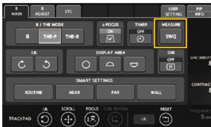
1. While the ultrasound image is live, press the B MAIN tab or the ELST MAIN tab to switch the touch panel to the B MAIN or ELST MAIN screen.
