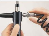
Attach the leakage tester to the venting connector on the endoscope.
