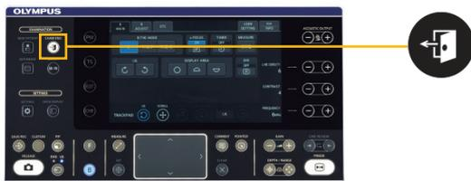
Press the EXAM END key on the keyboard to set the Ultrasound Center to the status shown in the following table.
