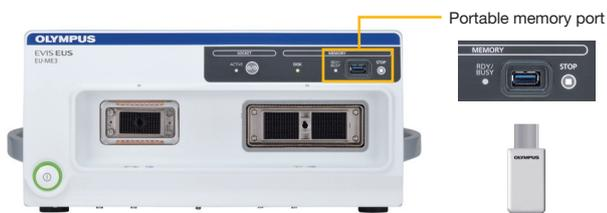
With the “OLYMPUS” logo on the portable memory facing up, push the portable memory into the portable memory port until it cannot go any further.
