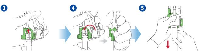
Put the distal-end of the endoscope inside the green cover with the back side surface viewable Shut the white cover and the green cover with a snap.
