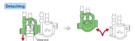
Open the white cover and the green cover to detach MAJ-2319 from the endoscope. Then separate the white cover and the green cover.
