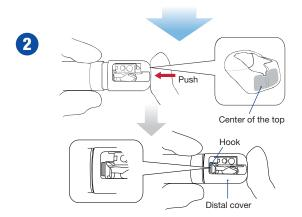
2. Put your finger onto the center on the top of the distal cover and push the top of the distal cover straight onto the distal end of the endoscope until the hook of the distal ring is completely visible within the opening of the distal cover.
