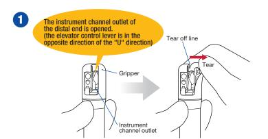
Hold the gripper of the distal cover and tear the top of the distal cover along the tear off line.
