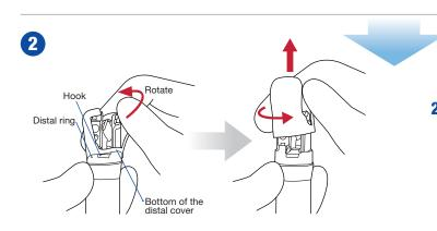
Keeping the gripper apart from the distal end, rotate the distal cover in the direction of the arrow as shown above until the bottom of the distal cover is removed from the hook of the distal ring to detach the distal cover.
