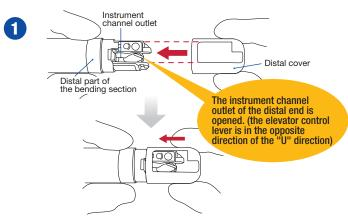
1. Gently hold the distal part of the bending section and the distal cover. Align the opening side of the distal cover with the lens side of the distal end of the endoscope.
