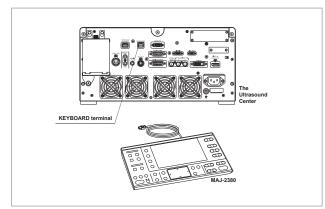
Reconnect the EU-ME3 keyboard to the KEYBOARD terminal on the back of the EU-ME3.
