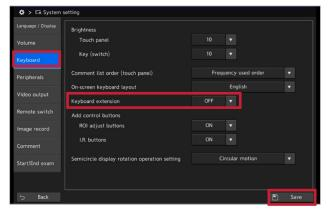
Press the Settings button on the keyboard and then choose System setting > Keyboard. Turn **OFF** the **"Keyboard extension"** function and press **Save**.
