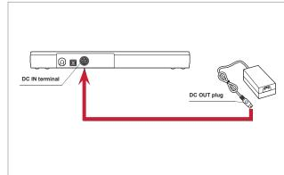
If not already connected, connect the AC adapter (MPU16A-102) to the EU-ME3 keyboard and plug the AC adapter into a power source.
