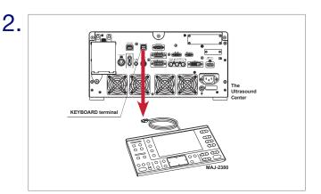
Turn **OFF** the EU-ME3. Disconnect the keyboard cable from the back of the EU-ME3.
