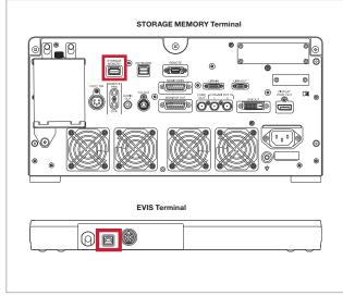
Plug a USB-AB cable (MAJ-1711, MAJ-1918 or equivalent) into the EVIS Terminal on the EU-ME3 keyboard and the STORAGE MEMORY Terminal on the back of the EU-ME3.
